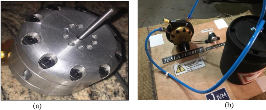
Fig 3. (a) Tesla Turbine Assembly; (b) - Turbine set onto a test rig
