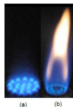
Fig. 3 Top view of: (a) perforated Bunsen flame with secondary Bunsen open tip flame, \phi = 0.72 ; (b) Triple flame with cellular flame, \phi = 1.61
