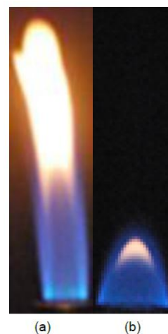
Fig. 9 Secondary Bunsen Flame Open Tip: (a) coconut oil with glycerol \phi=1.14 , (b) oil without glycerol \phi=1.24
