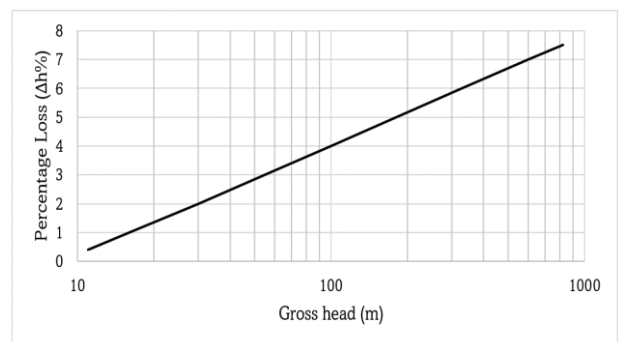
Fig. 3 - Percentage hydraulic loss in a hydroelectric installation as a function of gross head (Leite, 2020).
