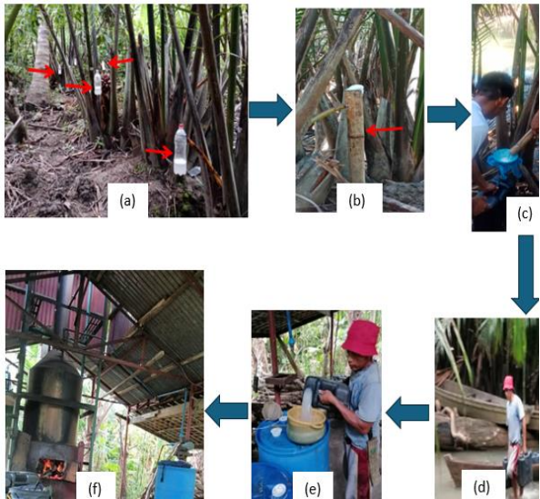
Fig 2. Nipa Bioethanol Production: (a) Sampling; (b) Bamboo Sap collection; (c) Sap Collection; (d) delivery to facility; (e) further storage; (f) distillation
