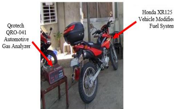
Fig 4. Emission testing process and test vehicle
