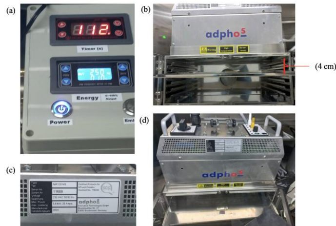
Fig 3. FIRA system used in the annealing of the PCBM ETL (a) control unit (b) annealing chamber (c) system specification (d) FPSC being annealed in the chamber
