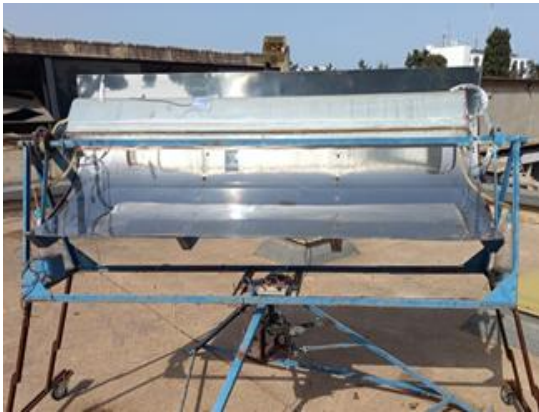
Fig. 3. Pictorial view of parabolic trough concentrator conventional solar still
