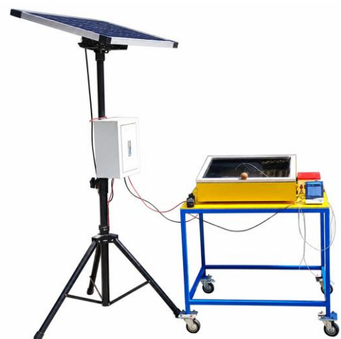
Fig. 2 3D views of ventilation direct solar dryer
