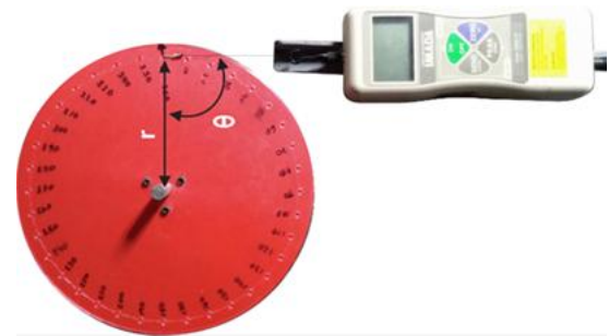
Fig 5. Experimental setup for measurement disk and dynamometer for torque measurements
