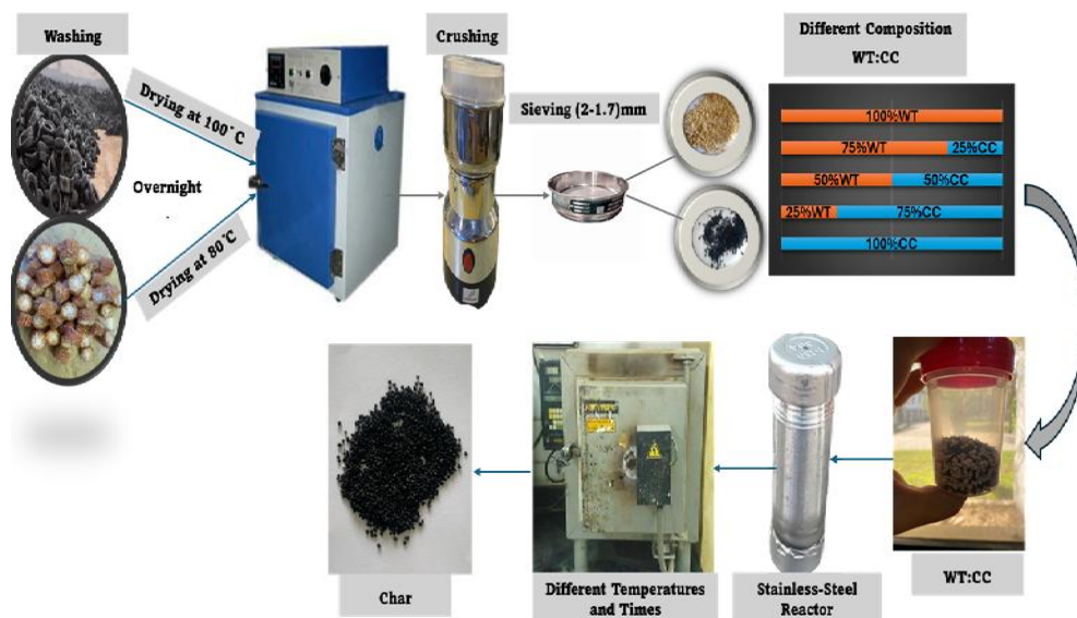
Fig. 1. Schematic diagram for char preparation
