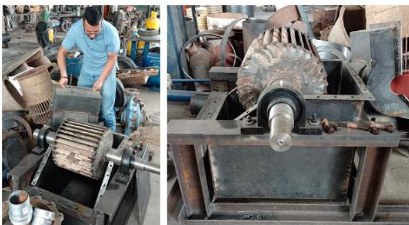
Figure 4. Presentation of turbine components: Rotor – Casing – Structure, in the metalworking manufacturing workshop.
