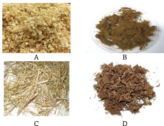
Fig. 3 Samples of processed and unprocessed plant material. A – Chopped pine wood; B – ALM from pine wood ( t_{st}=210\text{ }^{\circ}\text{C} ); C – Crushed wheat straw; D – ALM from wheat straw ( t_{st} =165\text{ }^{\circ}\text{C} ) *ALM, activated lignocellulosic mass
