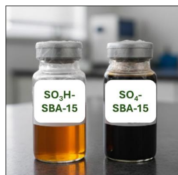
Fig. 6 Liquid products of the HAA reaction of 2-MF and MIBK using \text{SO}_3\text{H-SBA-15} and \text{SO}_4\text{-SBA-15} catalysts.
