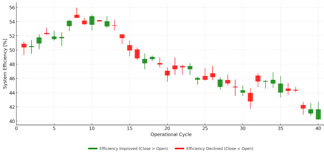
Fig. 10 Cycle-by-cycle efficiency variation of the hybrid PEMFC–battery propulsion system using candlestick representation, illustrating efficiency fluctuations, improvement and decline trends, and overall system stability under dynamic operating conditions
