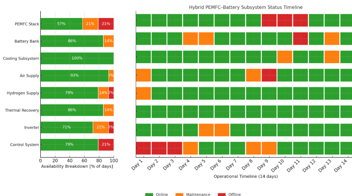
Fig. 13 Availability analysis of the hybrid PEMFC–battery system over a 14-day operation period, showing percentage distribution of Online, Maintenance. and Offline states (left) and daily subsystem status timeline (right). highlighting system reliability and maintenance patterns.
